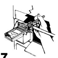
Secure coin-slide mechanism from inside the control panel using the 3/16" bolt and washer supplied. Install coin box.
